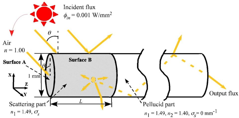
Figure 3. Numerical model of radiative transfer in optical fiber.
