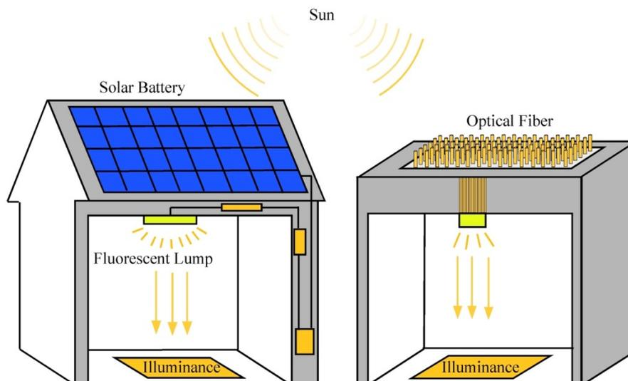
Figure 1. Schematic of indoor light guided from sunlight through optical fibers.
