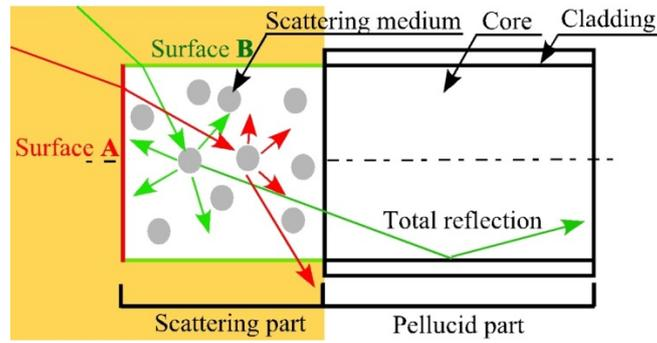
Figure 2. Schematic of optical fiber attached scattering medium at edge.
