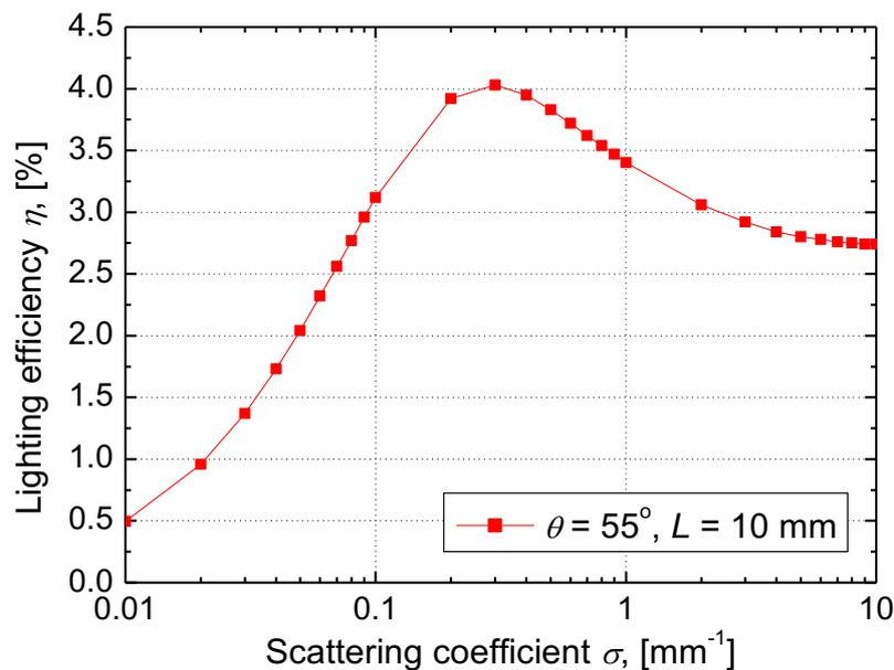
Figure 4. Effect of scattering coefficient on lighting efficiency when length of scattering media is 10 mm and incident angle of sunlight is  $55^\circ$
