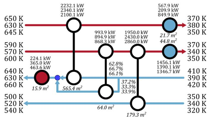
Figure 3. Optimal multiperiod HEN configuration for case study 1
