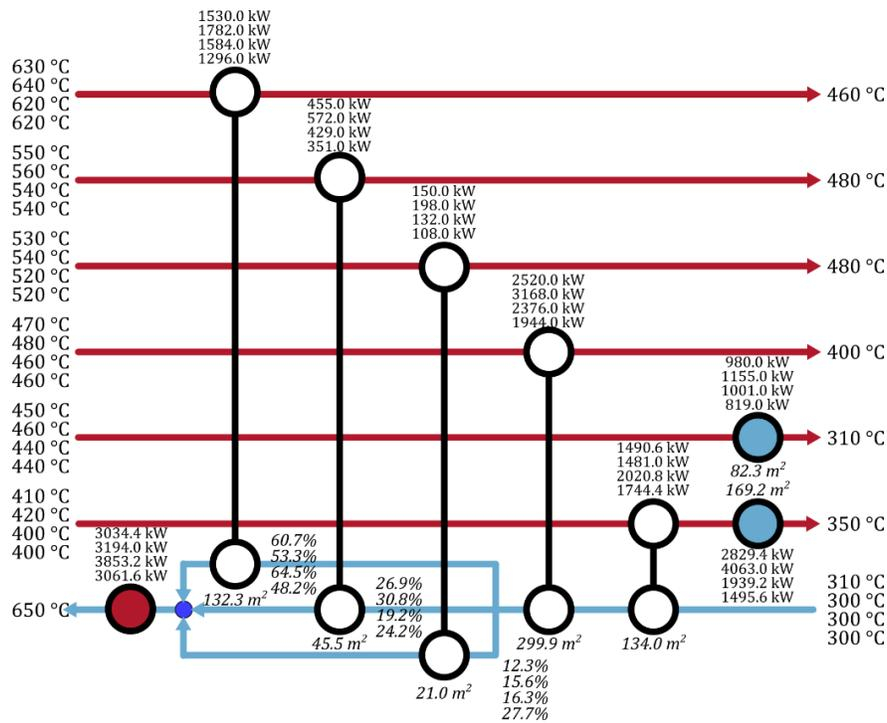
Figure 4. Optimal multiperiod HEN configuration for case study 2
