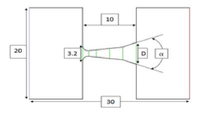
Figure. Geometry of the diode studied convergent / divergent (dimensions in mm)
