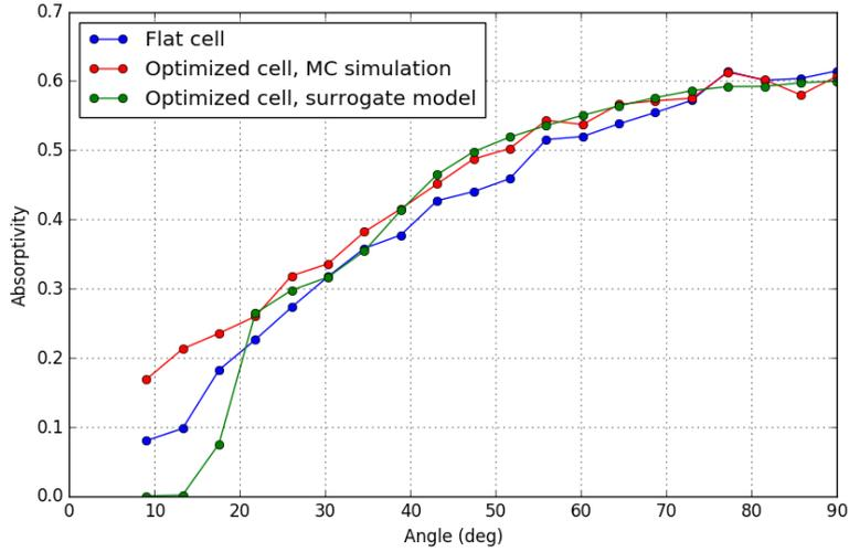
Fig. 7. Absorptivity versus incident angle for the 3 piece panel optimized using the surrogate model for full-day average radiation and the flat panel.
