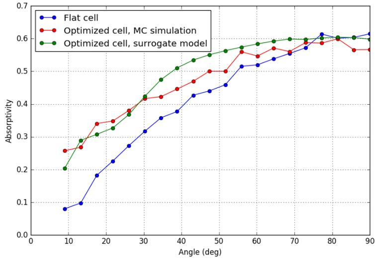
Fig. 6. Absorptivity versus incident angle for the 3 piece panel optimized using the surrogate model for half-day average radiation and the flat panel.
