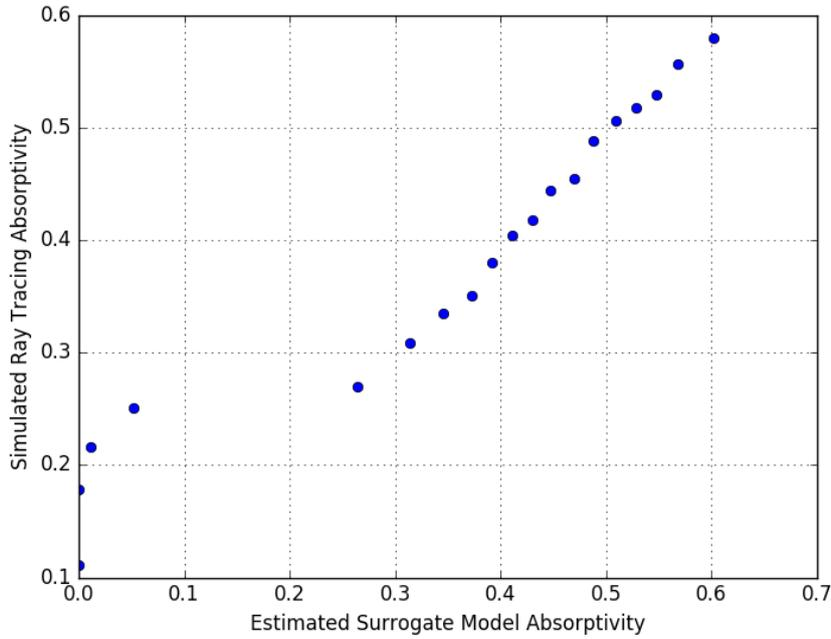
Fig. 5. Quantile bin-plot of estimated absorptivity for out-of-sample data using the surrogate model versus the accurate MC based calculation of absorptivity.
