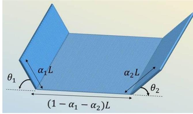
Fig. 1. Three-folded solar panel schematics.
