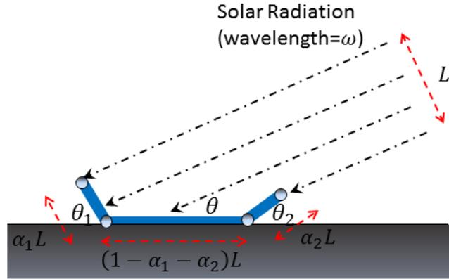
Fig. 3. Cross section demonstration of the 3 piece folded panel and incident ray of light.
