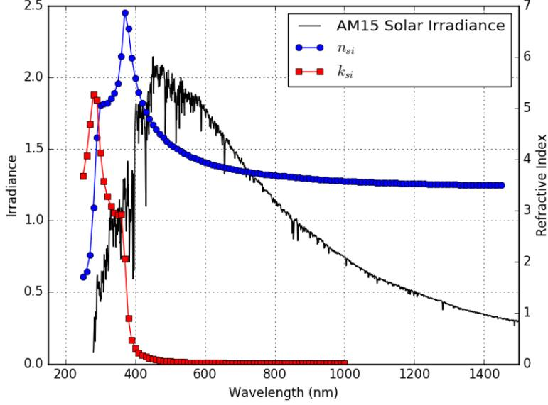
Fig. 2. Refractive index of silicon and AM1.5 solar irradiance.
